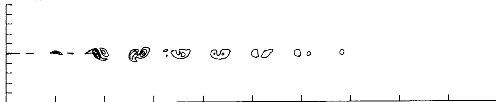
(D) INSTANTANEOUS KINETIC ENERGY OF THE OSCILLATORY MOTION ( \kappa = 3.0 TO 0.5 INTERVALS OF 0.5).
