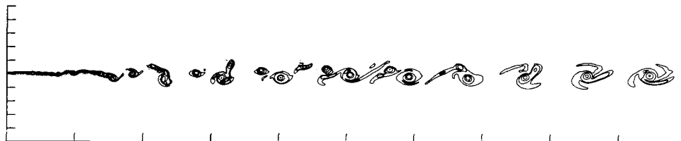
(B) INSTANTANEOUS VORTICITY FOR A FINE MESH CALCULATION (798 x 241 GRID POINTS). CONTOURS OF -500, -250, -100, -50, AND DASHED +50, +100.
