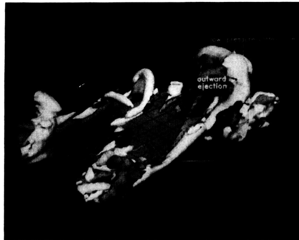
Figure 2. Turbulent flow-physics obtained from a full simulation of the Navier-Stokes equations. M_\infty = 0 , Re_\theta = 670 .
