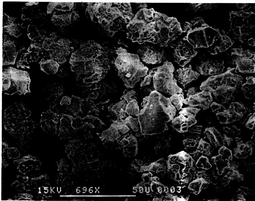
Figure 38. Scanning electron micrograph of as-received powder having 15 mol% \text{TiO}_2 ( 15\text{T}_2 ).
