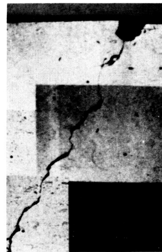
ACTUAL CRACK PROFILE IN INNER RACEWAY OF HIGH-SPEED BEARINGS
