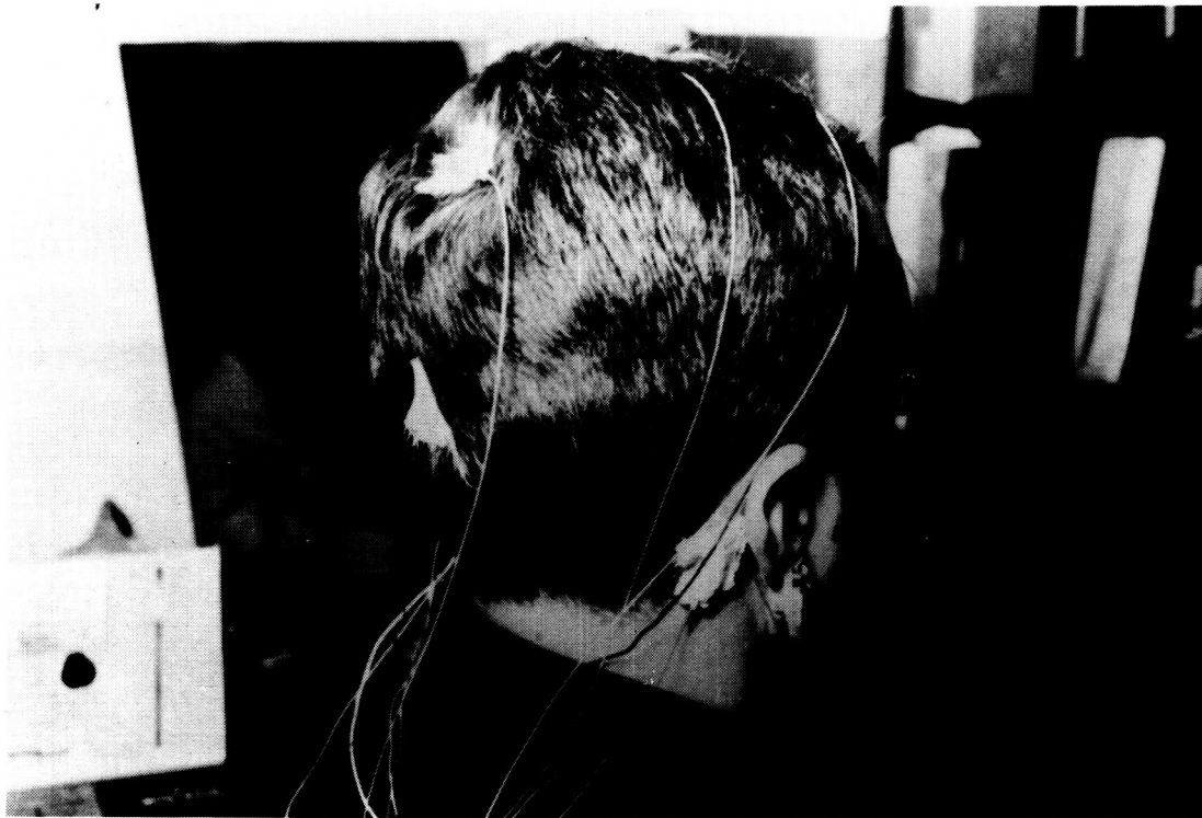
4. Attachment of event related potential (ERP) recording electrodes on a U. S. Navy sonarman
