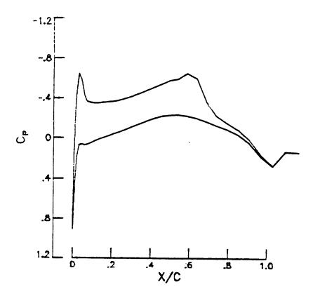
Figure 1a. ONERA M6 wing,  $M_{\infty}=.84,~\alpha=3.06,~96\times16\times16$  C-H mesh,  $\kappa^{(2)}=\frac{1}{4},~\kappa^{(4)}=\frac{1}{128},~{\rm station}=0.05.$
