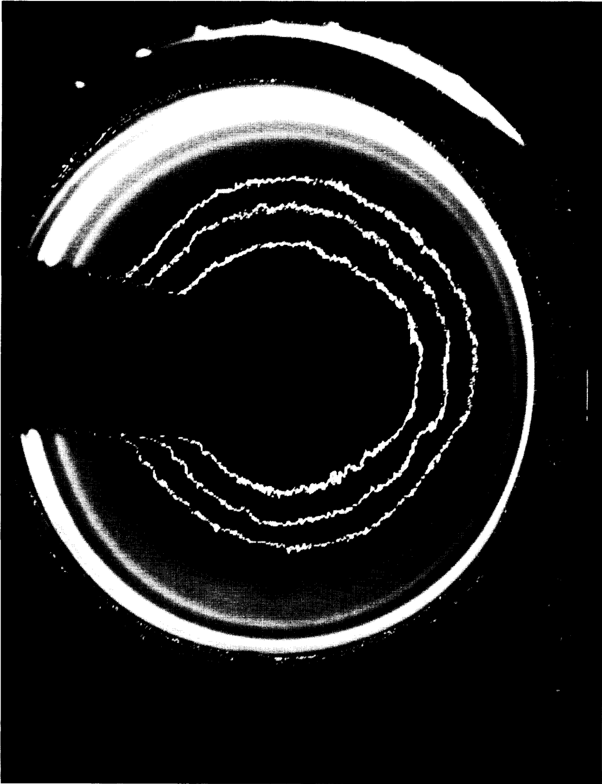
Figure 9 Isotherm representation after application of a two dimensional low pass filtering convolution utilizing a 3 \times 3 convolution kernel. Note the reduction in high spatial frequency noise resulting in a more coherent representation of the isotherms.
