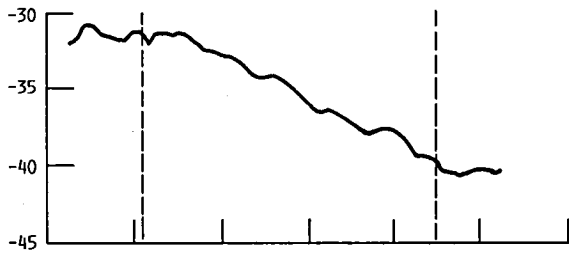
(a) TEST R1.0. TWT OPERATING POINT, LINEAR; GAIN VARIATION OVER 330 MHz, 8.3 dB.
