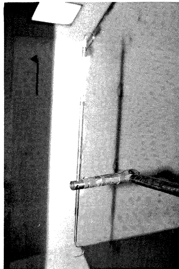
Figure 3d. Close up of the five-tube-probe as mounted behind the model.
