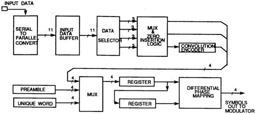
Fig. 5. Encoder block diagram.
