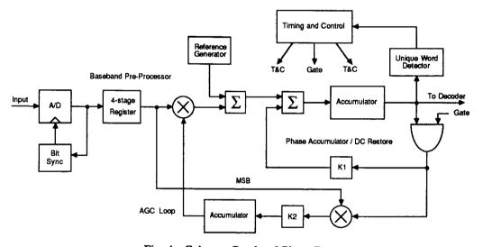
Fig. 4. Coherent Baseband Phase Detector.
