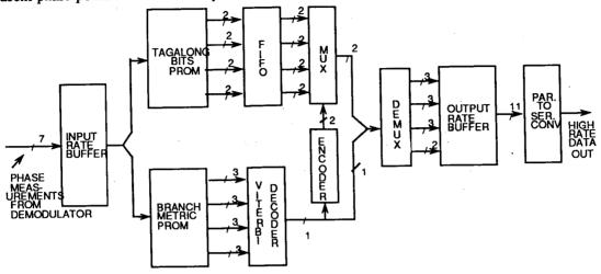
Fig. 6. Decoder block diagram.
