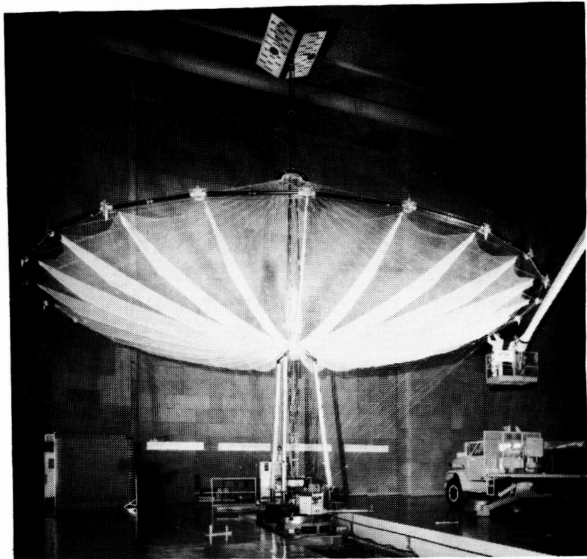
Fig. 1. 15-meter antenna in Martin Marietta Near Field Facility
