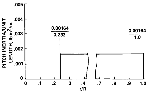
Fig. 12 Calculated model blade-pitch inertia per unit length (computed).
