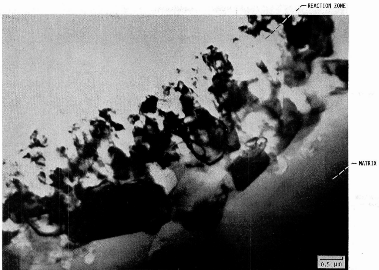
(A) SMALL CRYSTALLITES WITHIN REACTION ZONE.
