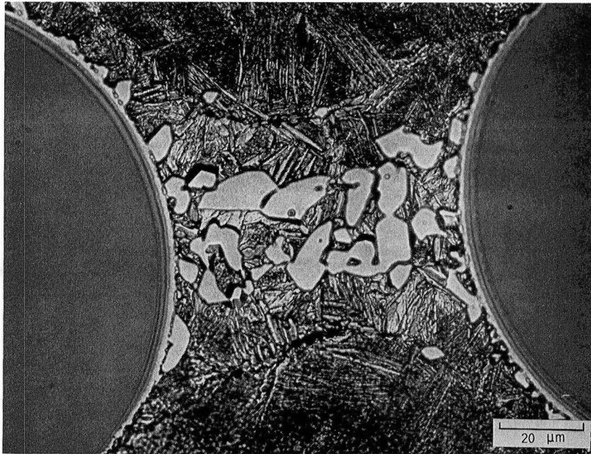
FIGURE 6. - LARGE, WHITE PARTICLES OF TiC AND \alpha - \beta LAMELLAR STRUCTURE FORMED FROM Ti WIRE WOVEN BETWEEN FIBERS PRIOR TO CONSOLIDATION (SPECIMEN POLISHED AND ETCHED).
