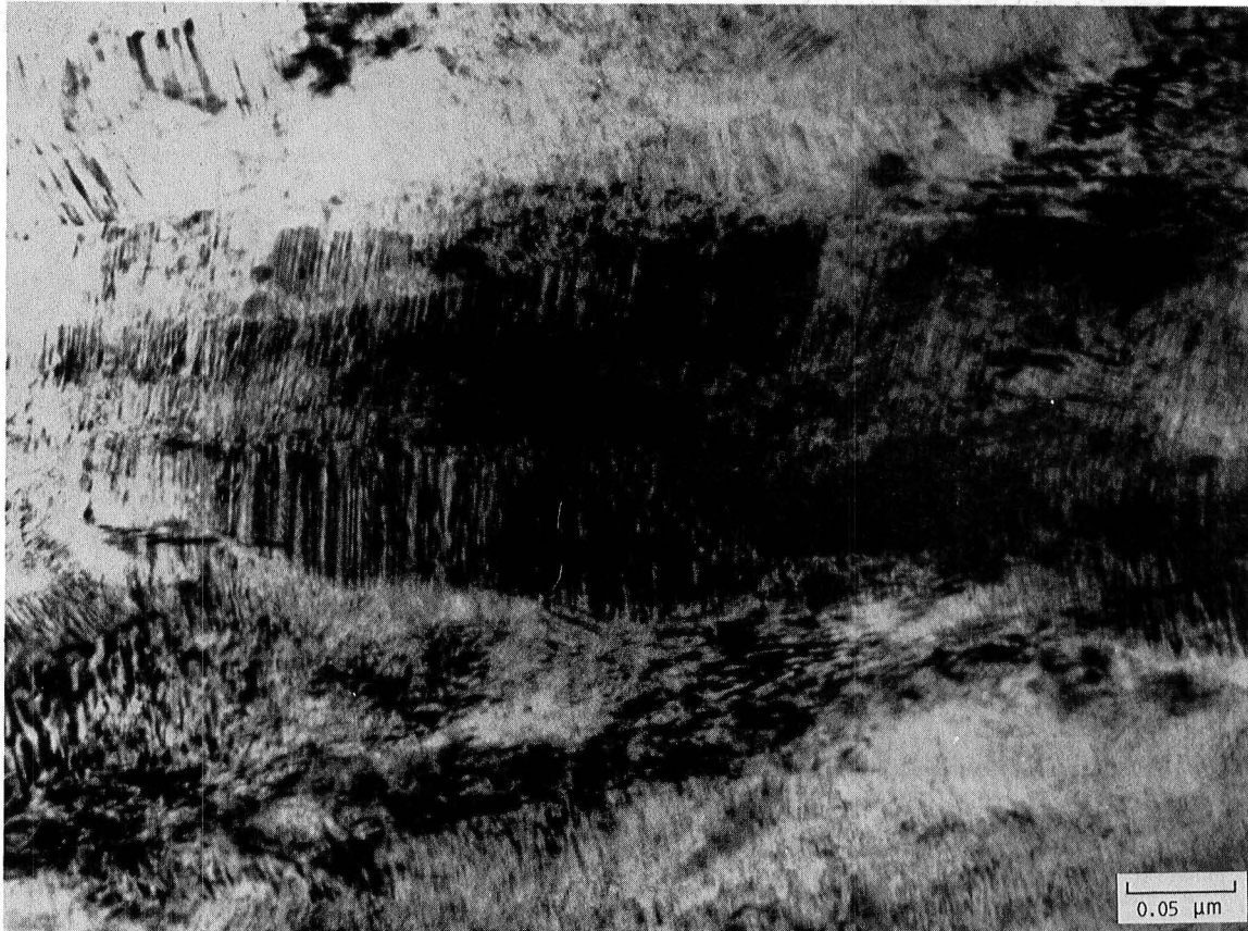
(A) LARGE, ELONGATED GRAINS CONTAINING STACKING FAULTS.
