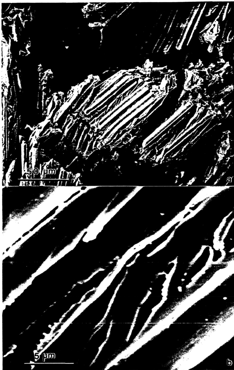
Fig. 12 Details of the shear crippling zone and matrix microcracking.
