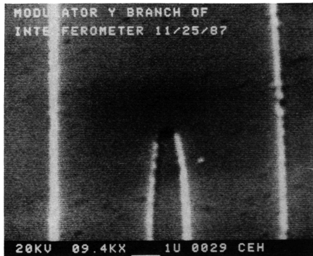
FIGURE 3. - "Y" BRANCH OF MACH-ZEHNDER INTERFEROMETER. GAP BETWEEN BRANCHES IS APPROXIMATELY 1\ \mu\text{m} AT IT'S NARROWEST POINT.
