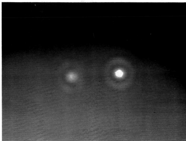
FIGURE 5. - OUTPUT OF MODULATOR CLEAVED MIDWAY ALONG INTERFEROMETER. EACH OF THE INTENSITY PEAKS LIES UNDER ONE OF THE PARALLEL WAVEGUIDES.
