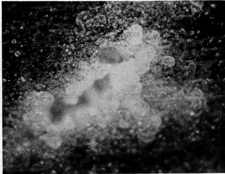
FIGURE 4. - VIEW OF DAMAGE FOR PMR-15 WITH 0.35 \text{ J/cm}^2 PER PULSE.
