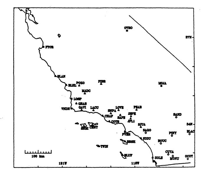
Figure 4. GPS network for central and southern California, showing regional fiducial sites ( < ), sites of the primary network (  $\Delta$  ), and VLBI sites observed by the NGS (  $\Diamond$  ).
