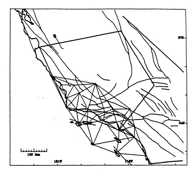
Figure 1. Network of sizes occupied during our initial experiments in June 1986, December 1986, and January 1987. The large pentagon outlines the "fiducial" sizes whose coordinates are well-known from VLBI and/or SLR observations.
