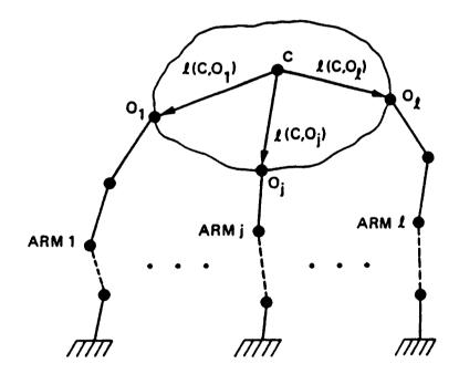
Fig. 2.1  $\ell$  Manipulators grasping a common object
