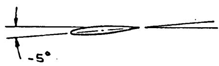
TIP CHORD (B.P. 542.0) 0012 - 64 SERIES AIRFOIL
