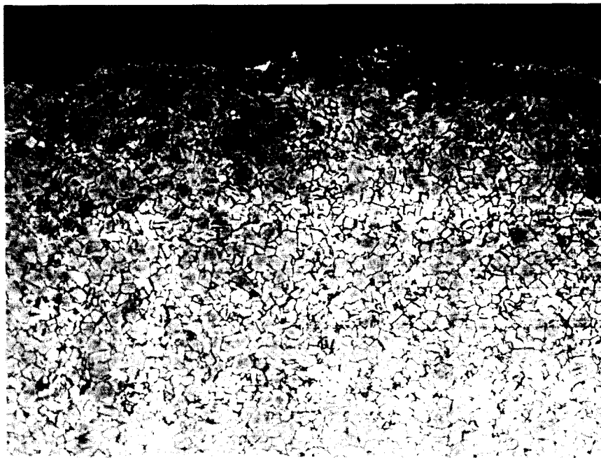
FIGURE 50. AFTER BOND TESTING. SPECIMEN NO. INT-7 WITH FG T-800 SPRAY DEPOSITED TRIBALLOY ON TYPE 718 INCONEL SUBSTRATE. EXAMPLE OF A LOWER BOND STRENGTH SPECIMEN SHOWING AREAS OF PULLED-AWAY DEPOSIT.
