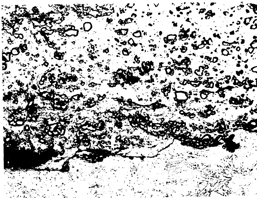
FIGURE 42. SPECIMEN NO. 17-9. CROSS SECTION WHERE COATING HAS MOSTLY PULLED OFF EXCEPT FOR VALLEYS IN THE PRE-SPRAY GRITTED SURFACE. ELECTROLESS NICKEL PLATED \text{FeCl}_3 ETCHANT.
