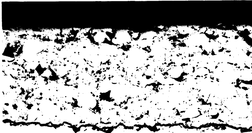
FIGURE 38. TUNGSTEN CARBIDE ON 17-4PH. NOTE THE INTIMATE BOND THAT IS FORMED WITH THE SUBSTRATE.
