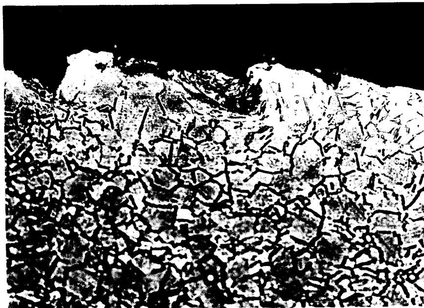
FIGURE 54. SPECIMEN INT-3. CROSS SECTION SHOWING AN AREA WITH SOME REMAINING ADHERENT FG T-800 DEPOSIT. ELECTROLESS NICKEL PLATED. \text{FeCl}_3 ETCHANT.
