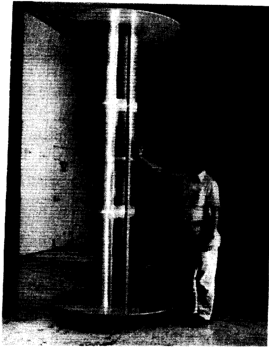
Figure 2. Two-dimensional test apparatus in the Langley 14 by 22 Foot Subsonic Tunnel. AH-64 cross section shown.
