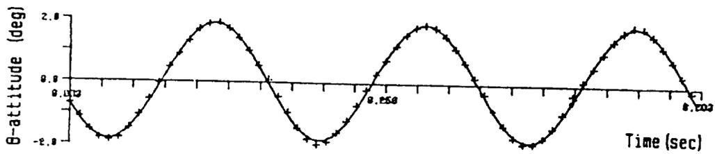
Fig.52 Model motion during a commanded 6Hz oscillating rotation about the y'-axis
