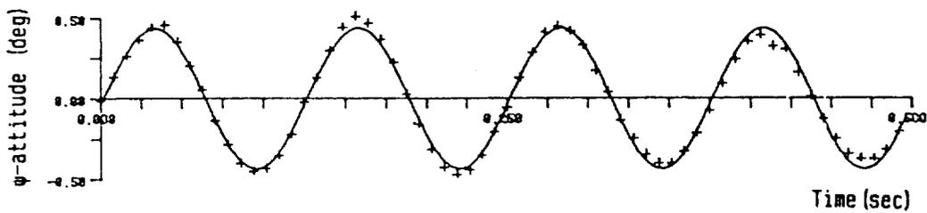
Fig.62 Model motion during a commanded 8Hz oscillation in the y'-direction
