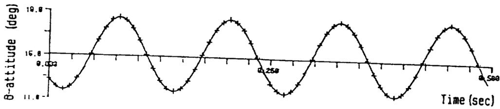
Fig.64 Model motion during a commanded 8Hz oscillation about the y'-direction (15 a-o-a)
