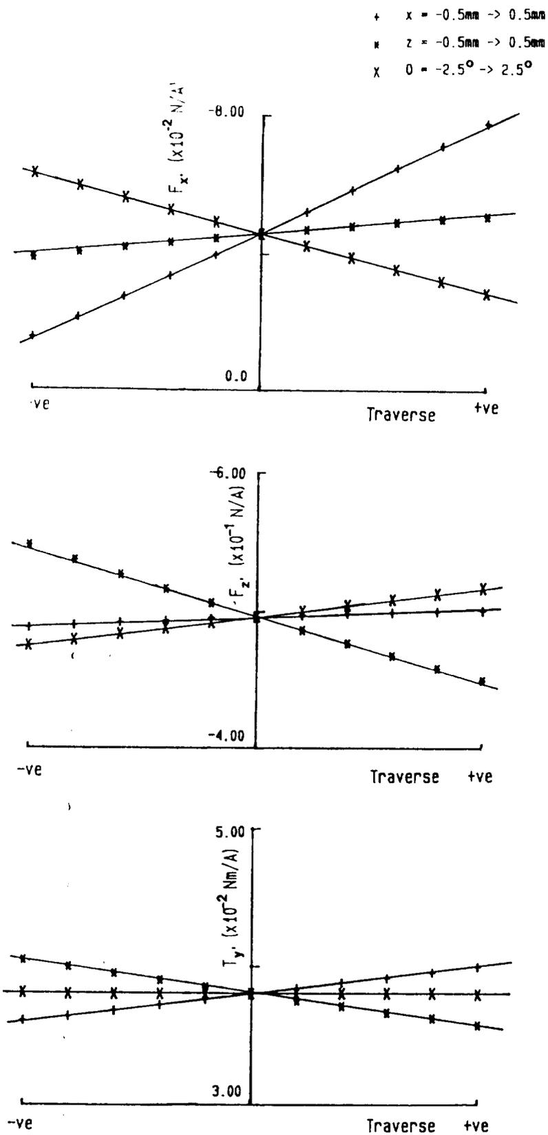
Fig.13 Variation in  $F_{x'}$ ,  $F_{z'}$ ,  $T_{y'}$  produced by e/m 1 during position and attitude changes
