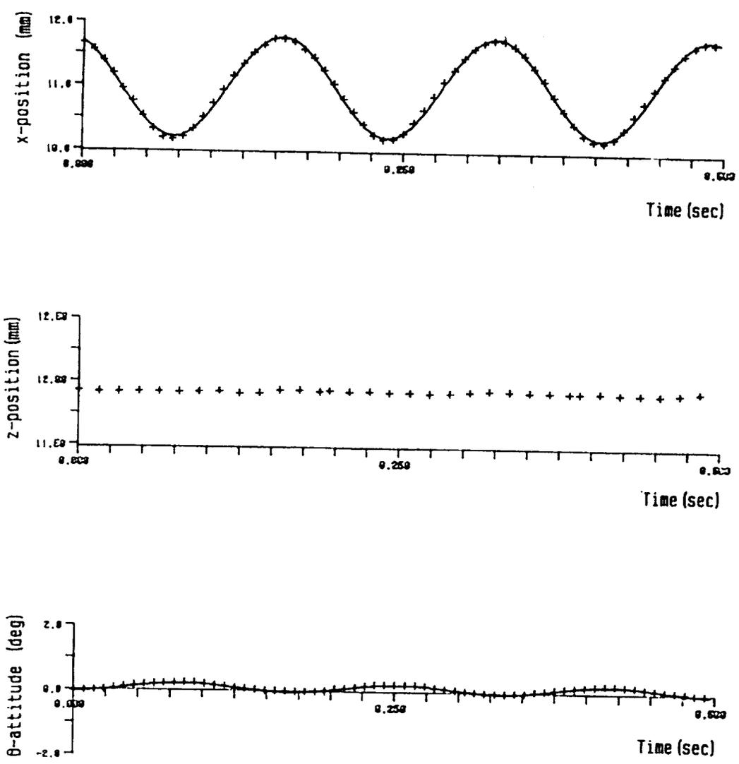
Fig.54 Model motion during a commanded 6Hz oscillation in the x'-direction
