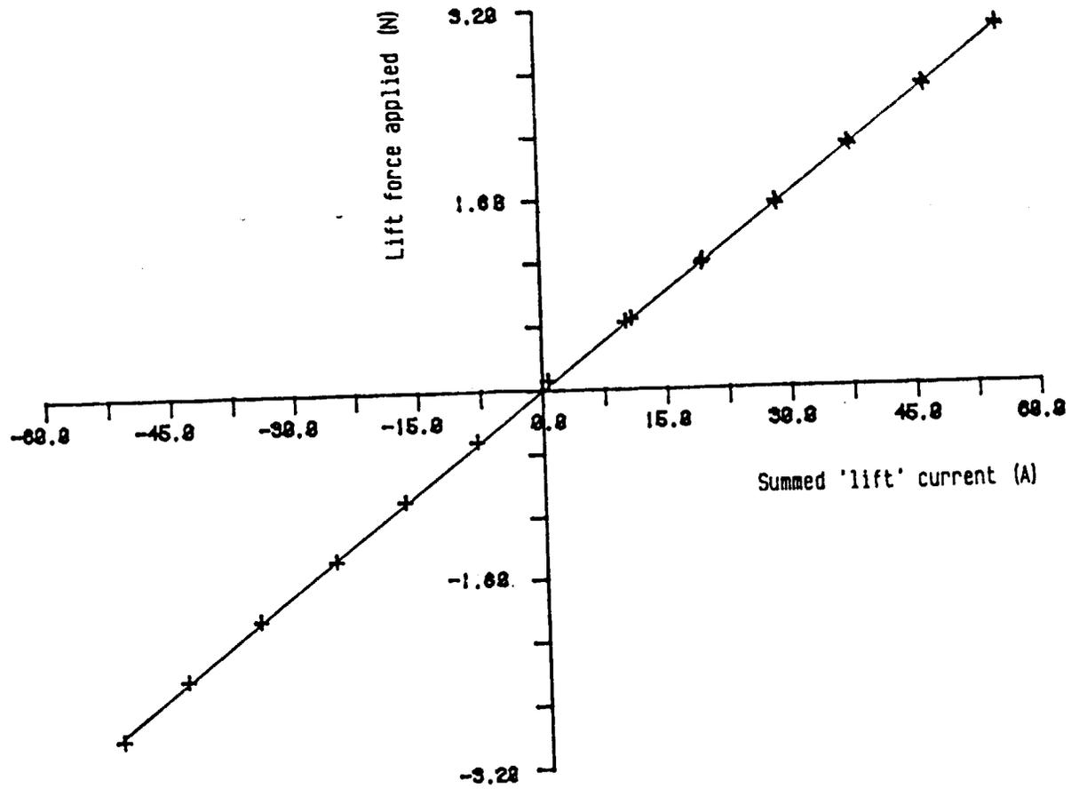
Fig.21 Static lift force calibration ( Samarium-cobalt model;  $0^{\circ}$  a-o-a)
