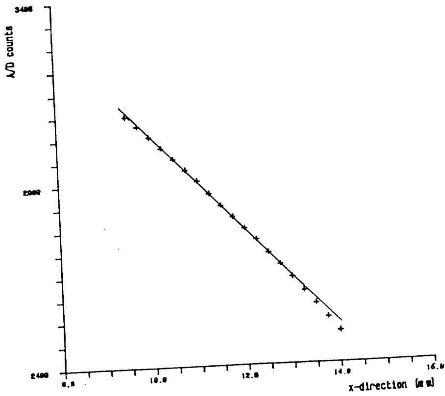
Fig.5.2 Axial sensor calibration ( 0 deg a-o-a )
