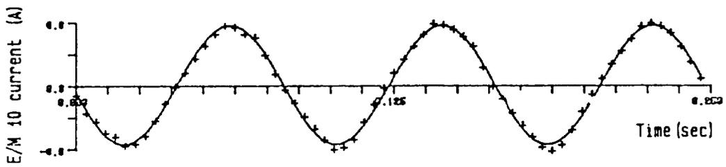
Fig.57 Current traces in e/m's 3,5,9,10 during a 12Hz oscillation in the z'-direction
