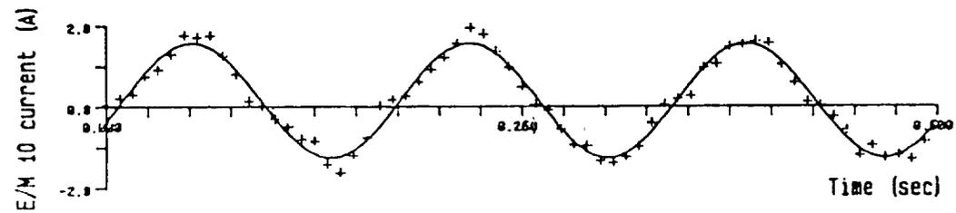
Fig.53 Current traces in e/m's 3,5,9,10 during a 6Hz oscillation about the  $y'$ -direction
