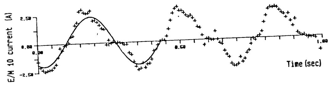
Fig.49 Current traces in e/m's 9 and 10 during a 3Hz oscillation in the x'direction
