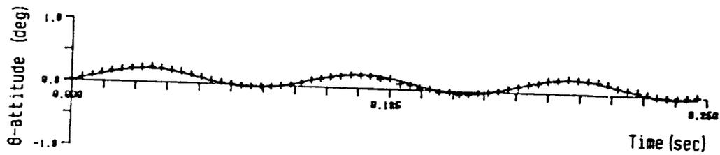
Fig.60 Model motion during a commanded 12Hz oscillation in the x'-direction
