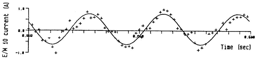
Fig.51 Current traces in e/m's 1, 7, 9, 10 during a 6Hz oscillation in the z'-direction
