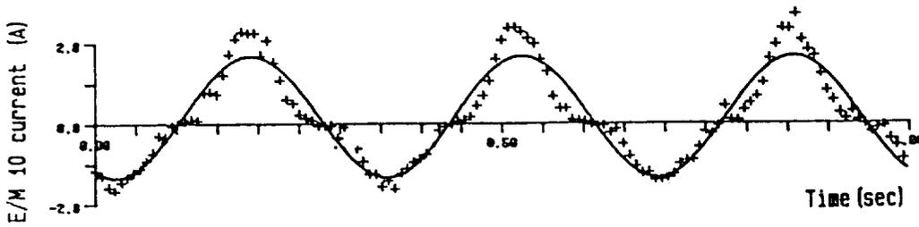
Fig.46 Current traces in e/m's 9 and 10 during a 3Hz oscillation about the  $y'$ -axis
