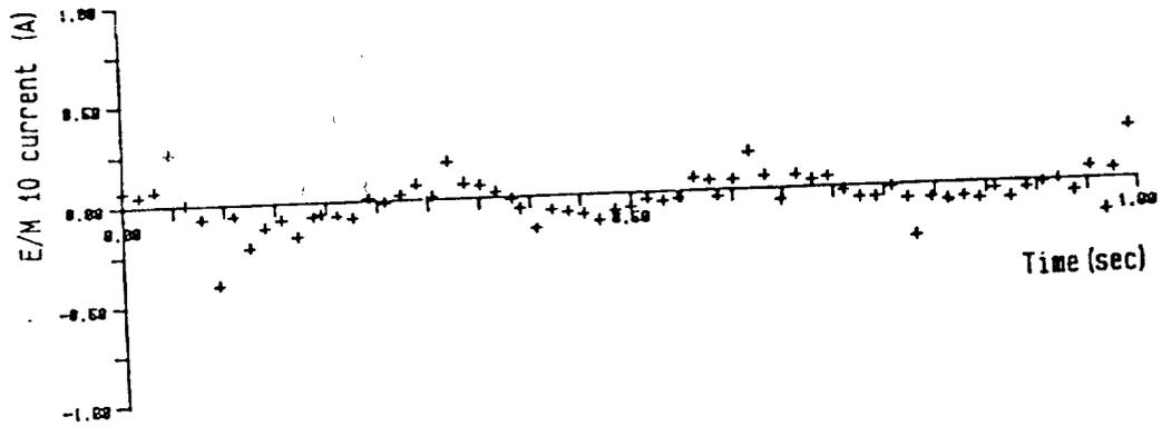
Fig.43 Current traces in e/m's 9 and 10 during a 3Hz oscillation in the z'-direction
