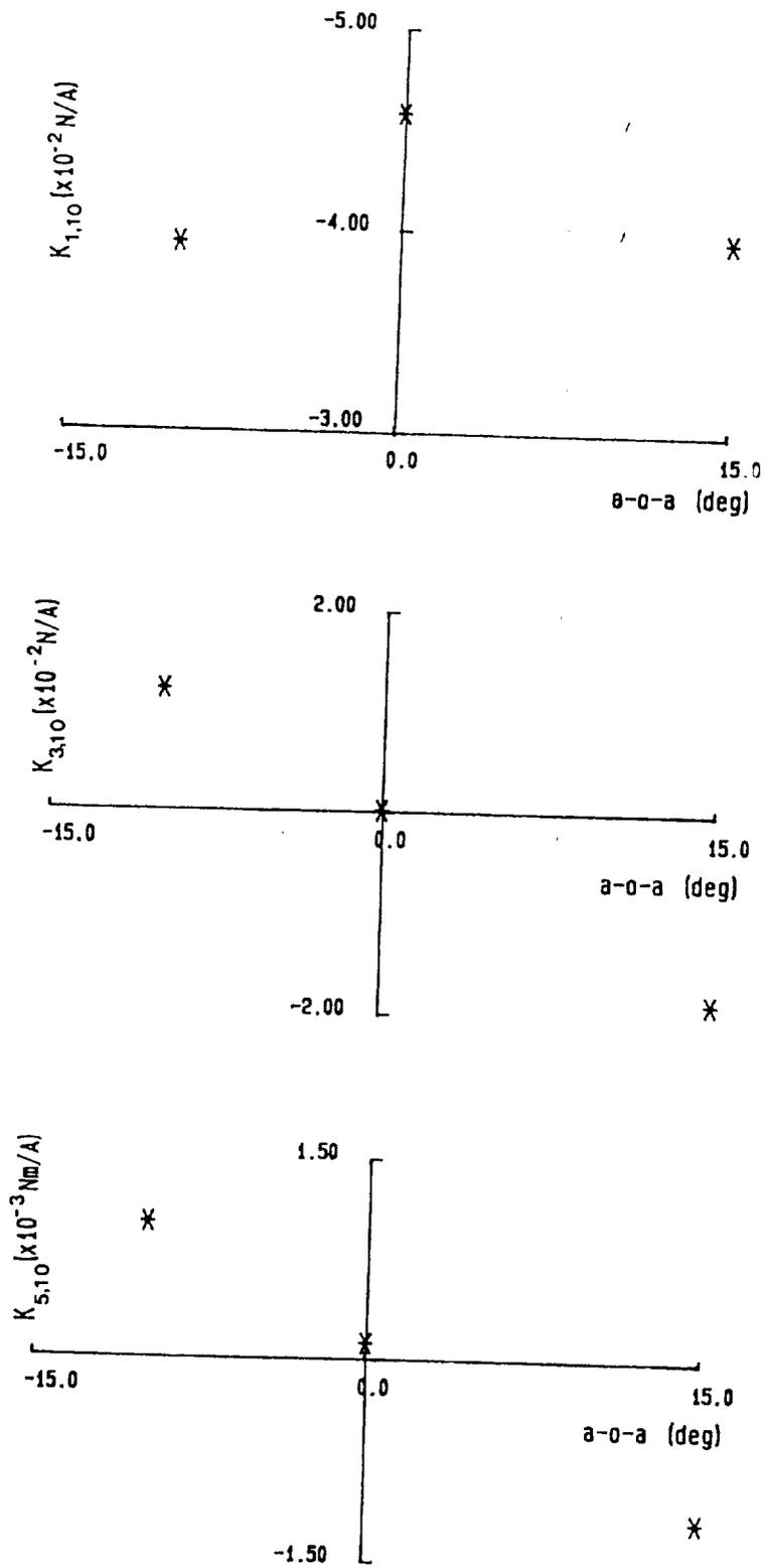
Fig.38 Force/Moment constants found by Static Calibration of Alnico model (e/m 10)
