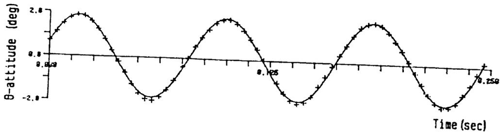
Fig.58 Model motion during a commanded 12Hz oscillating rotation about the y'-axis
