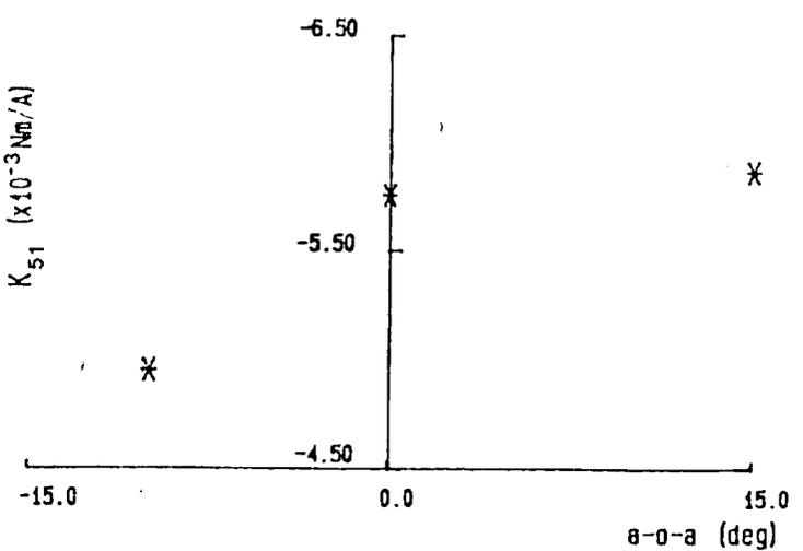
Fig.33 Force/Moment constants found by Static Calibration of Alnico model (e/m 1)
