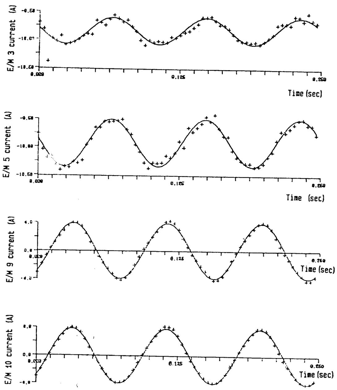
Fig.61 Current traces in e/m's 3,5,9,10 during a 12Hz oscillation in the x'-direction
