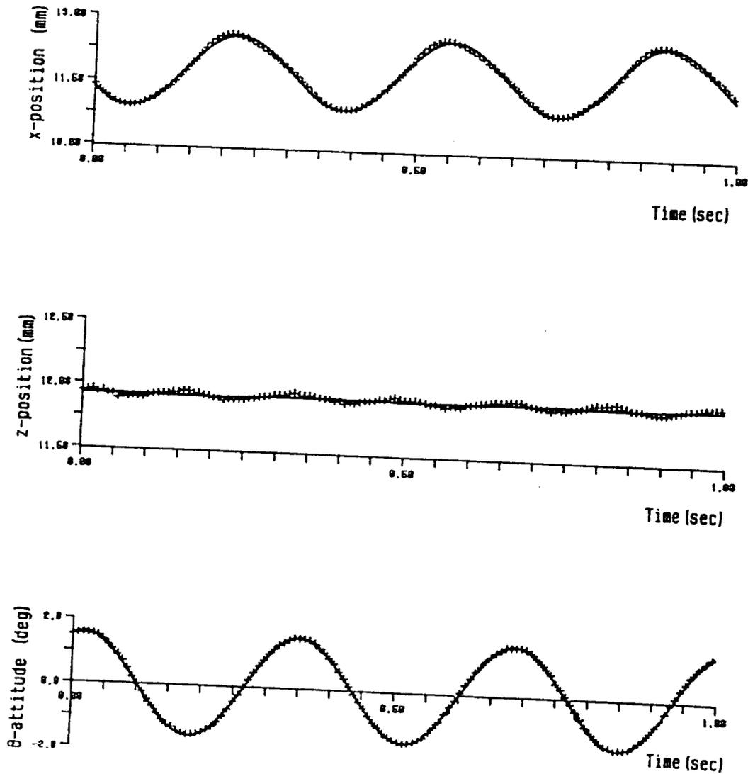
Fig.44 Model motion during a commanded 3Hz oscillating rotation about the y'-axis
