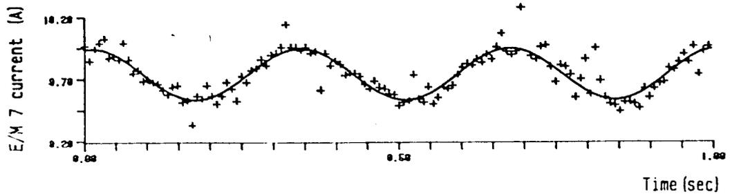
Fig.45 Current traces in e/m's 1,3,5,7 during a 3Hz oscillation about the y'-axis
