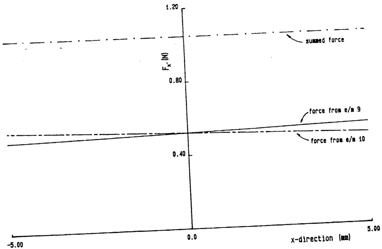
Fig.15 Variation in  $F_x$  produced by e/m<sup>9</sup> and 10 during a traverse in the x-direction
