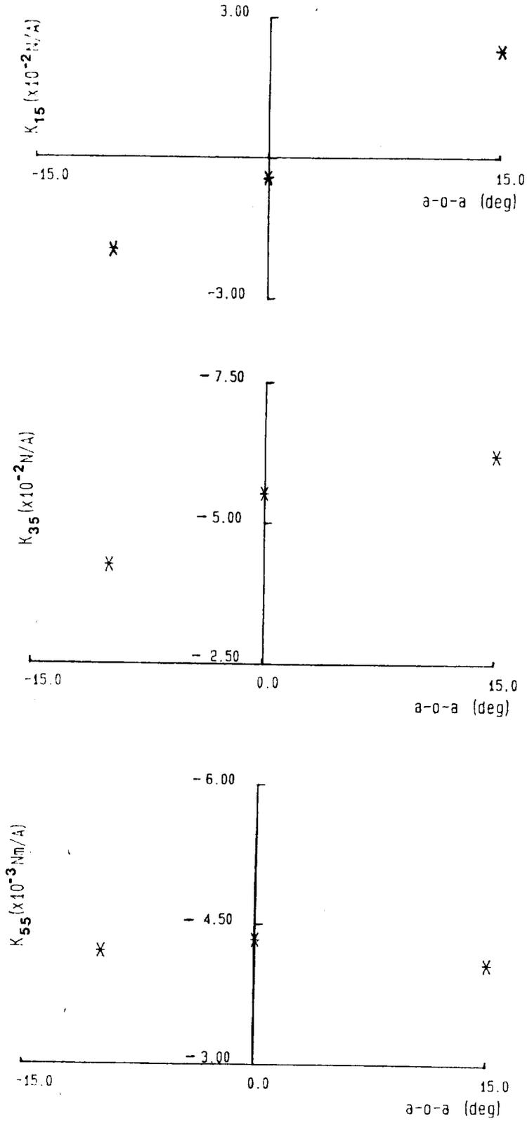
Fig.29 Force/Moment constants found by Static Calibration
