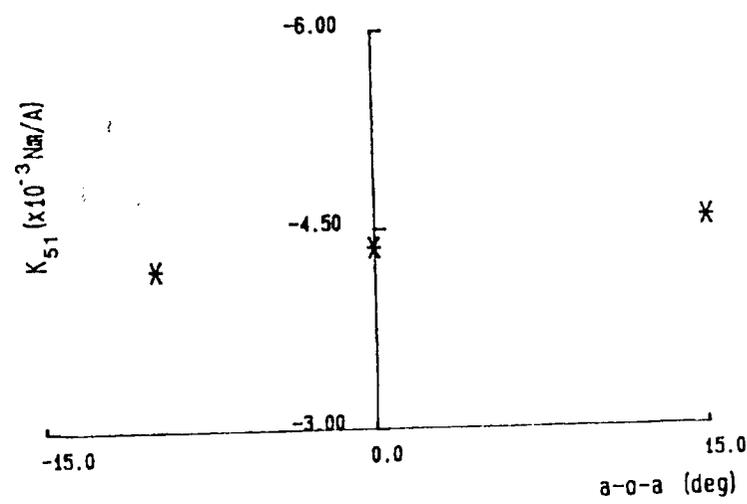
Fig.27 Force/Moment constants found by Static Calibration of Samarium-Cobalt model (e/m 1)
