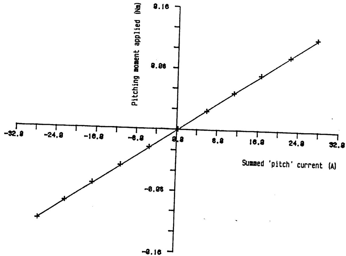
Fig.22 Static pitching moment calibration ( Samarium-cobalt model; 0° a-o-a)
