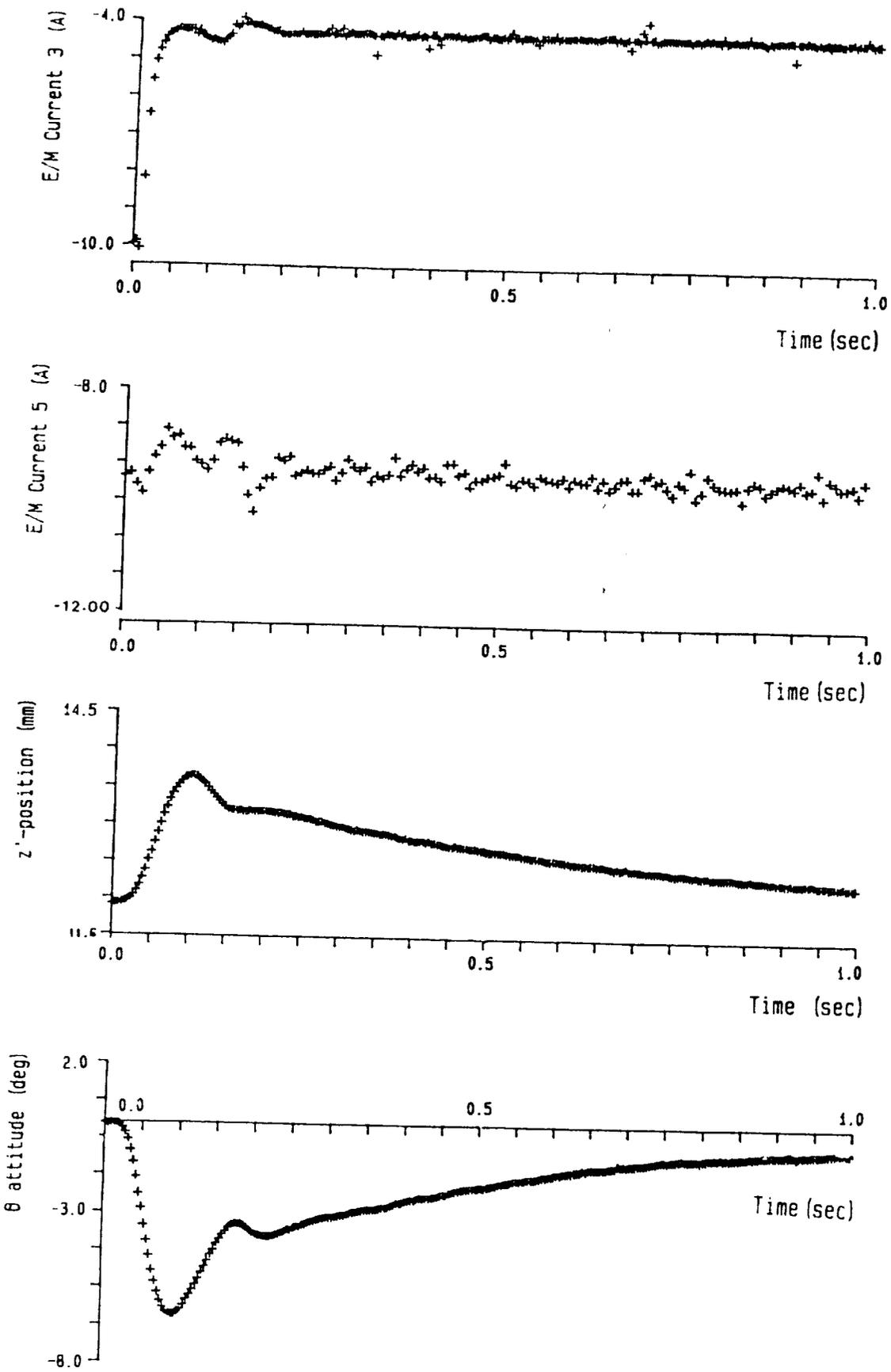
Fig.72 Response to a step in electromagnet current 3
