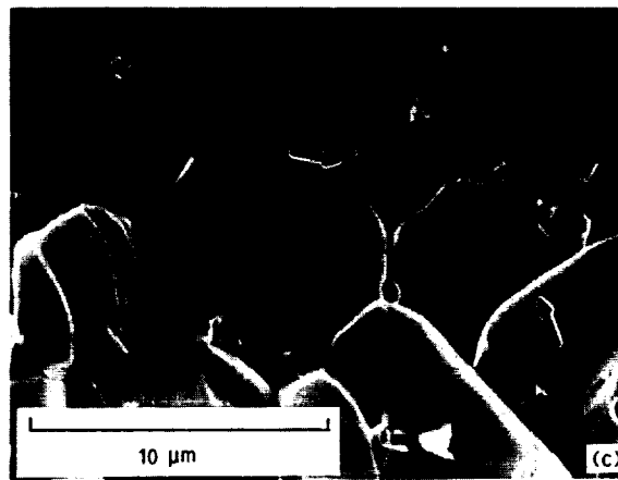
(c) PREFERENTIAL GRAIN BOUNDARY ATTACK AHEAD OF PIT IN (B).
