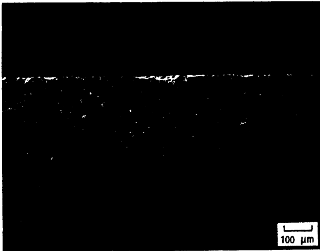
(a) OVERALL VIEW. (b) ENLARGEMENT OF CORROSION SCALE AND BUBBLES AT ORIGIN. FIGURE 27. - FRACTURE ORIGIN FOR SSN ( Al_2O_3, Y_2O_3 ) + Na_2SO_4/O_2 CORRODED AT 1000\text{ }^\circ C FOR 48 HR.
