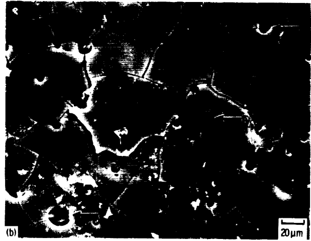
(b) WATER LEACH REVEALS BUBBLES AND PORES IN THE SILICA LAYER.
