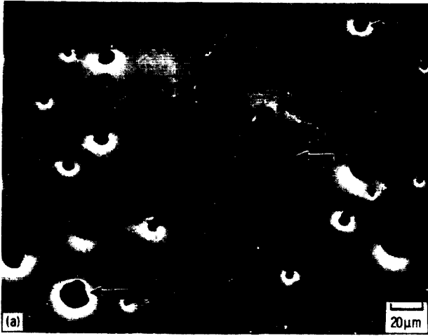
(a) AS-CORRODED SURFACE SHOWS BUBBLES AND PORES IN THE SILICATE LAYER.
