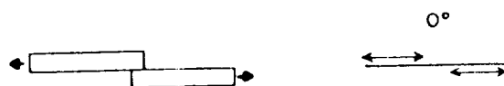
Figure C-1. - Schematic drawings of wood specimen geometry and loading, showing the relationship between glue line, grain direction, and loading.
