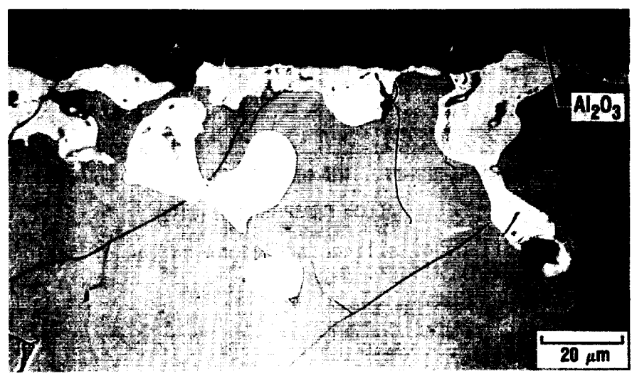
Figure 11 - Electron micrograph (back scatter) of Nb-40Al-8Cr-1Y oxidized at 1400^{\circ}C showing an increased scale thickness and grain growth.
