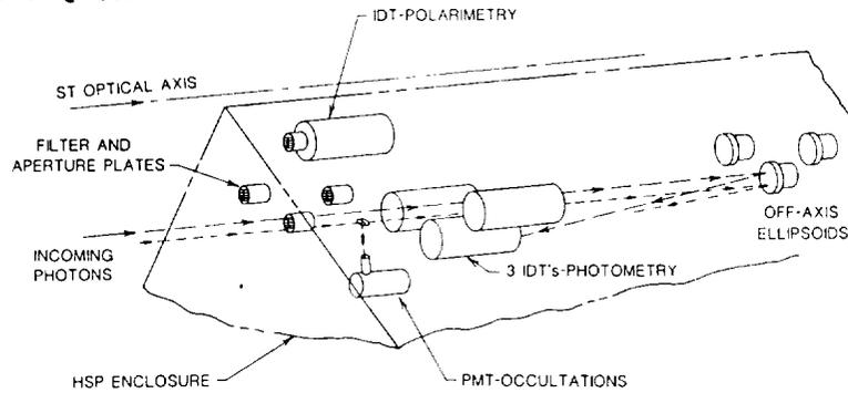
**Figure 1. Schematic Diagram of HSP Optics and Detectors
