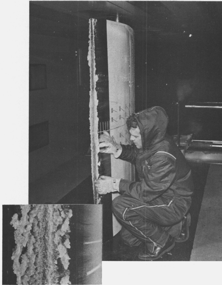
FIGURE 2. - THE AIRFOIL ICING PROBLEM.
