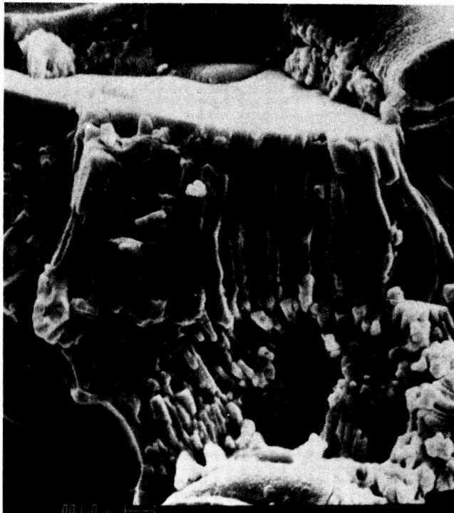
After 9000 Oxidation Cycles to 1010°C
