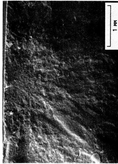
(b) \beta -SiC(1): \sigma_f = 745 MPA; 4 WT% C.
