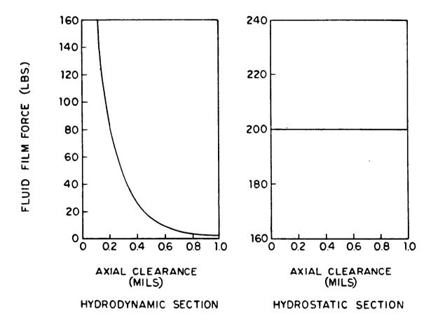
Figure 1.9: Hybrid Gas Seal F-h Curves - Hydrodynamic and Hydrostatic Components
