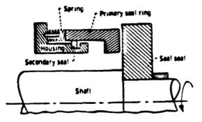
Figure 1.2: Schematic Diagram of a Face Seal
