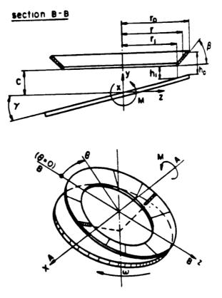
Figure 1.6: Face Seal with Angular Misalignment and Coning
