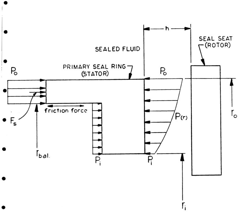
Figure 1.3: Force Diagram on a Stator
