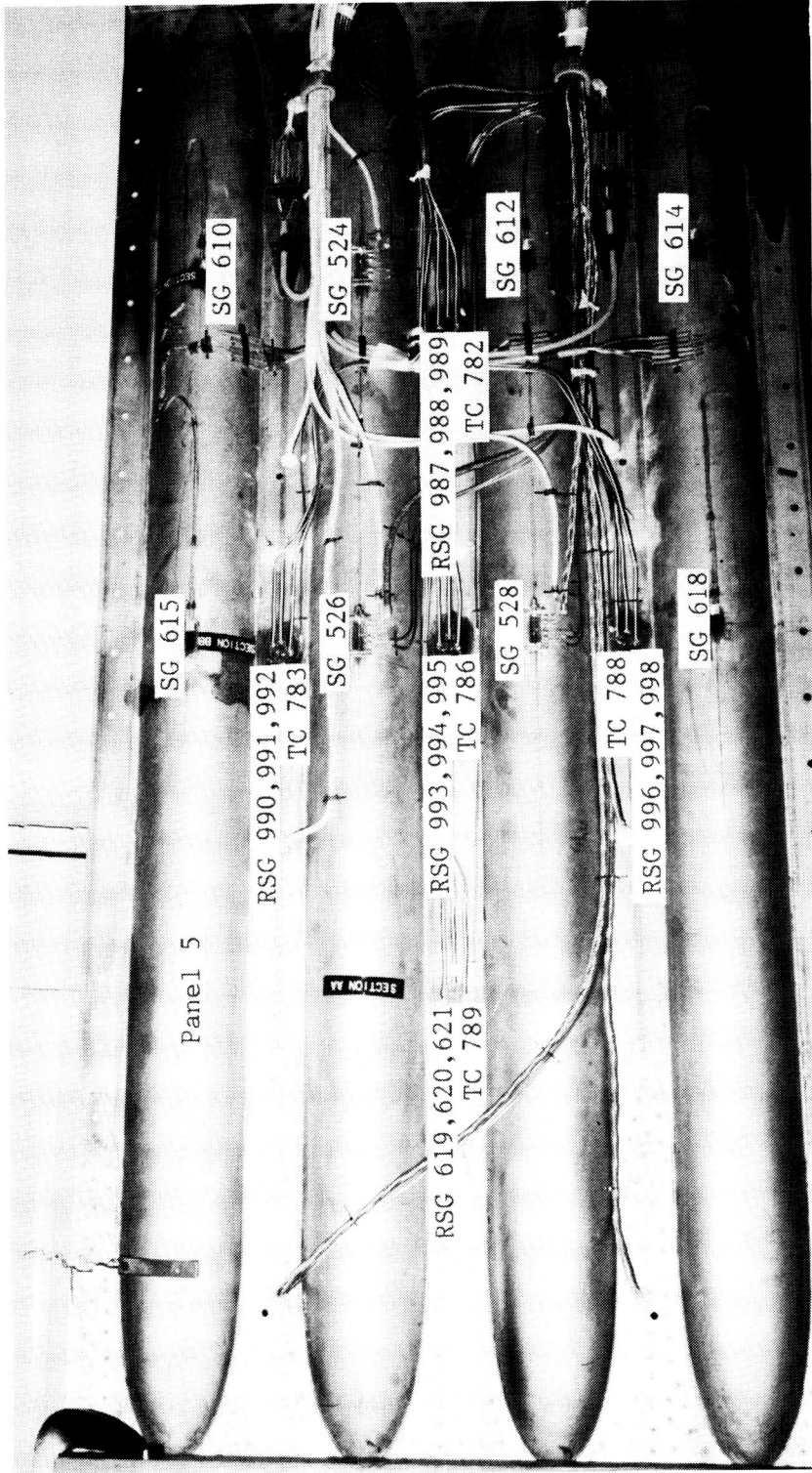
L-86-356 Figure 17. Strain gage and thermocouple (TC) instrumentation on outer (lower) surface of test panel 5.
