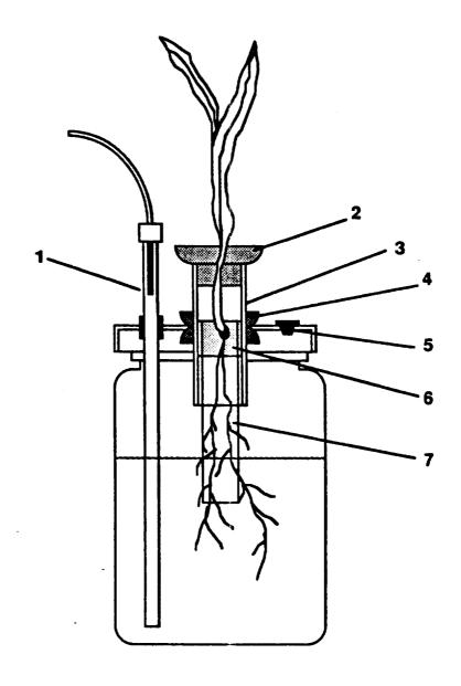
Figure 1. Vertical section of the glass hydroponic culture vessels designed for these experiments. Vessel volume is 500 ml. Vessel is cylindrical with a diameter of three inches. Key to diagram: 1 - aeration tube, 2 - foam plug, 3 - glass cylinder, 4 - foam gasket, 5 - injection port, 6 - foam seed holder, 7 - filter paper wick.
