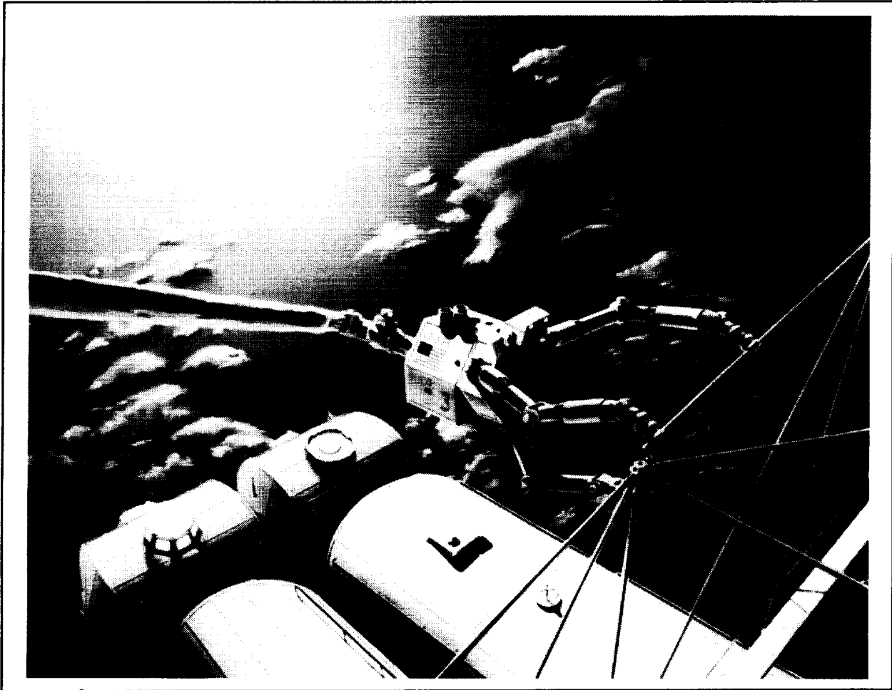
Figure V-8. Flight Telerobotic Servicer Performing an Assembly Task
