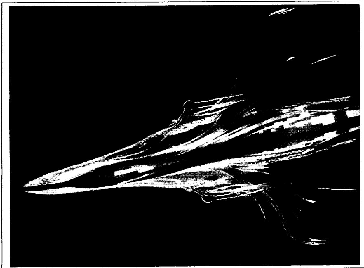
Figure VIII-1. Computer Generated Flowfield About an F-16 Aircraft
