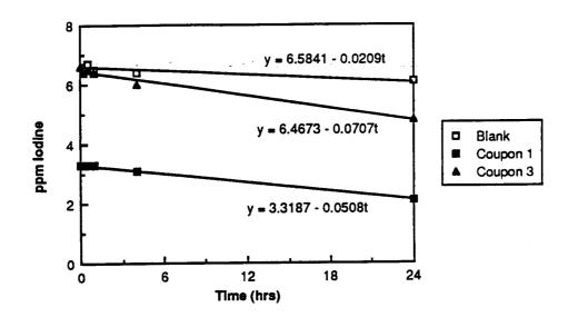
Figure 2a.- Iodine sorption by Viton A. First exposure with  $1" \times 2"$  coupons.
