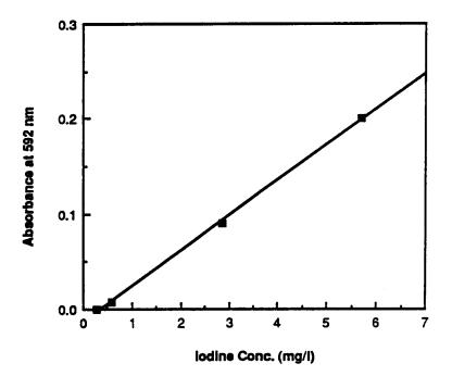
Figure 1.- Calibration curve for iodine analysis by the leuco crystal violet method using a 1.0 cm pathlength at 592 nm.
