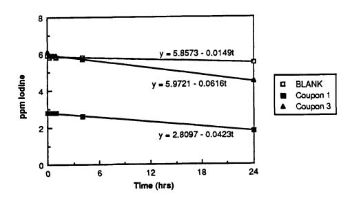
Figure 3a.- Iodine sorption by Viton A. Second exposure with  $1'' \times 2''$  coupons.
