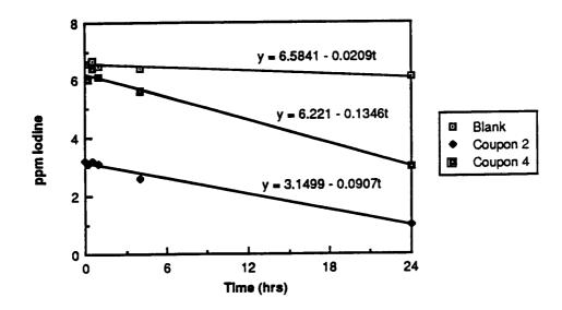
Figure 2b.- Iodine sorption by Viton A. First exposure with  $1.5'' \times 3''$  coupons.
