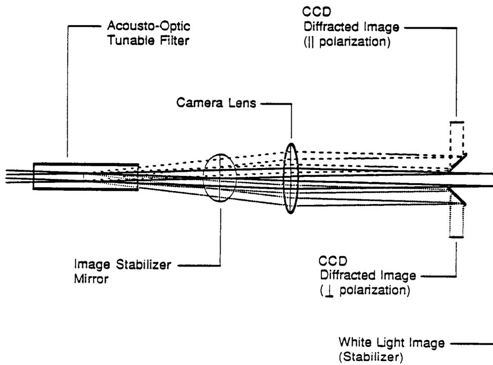
Figure 2. The analyzer section of the Imaging Vector Magnetograph.
