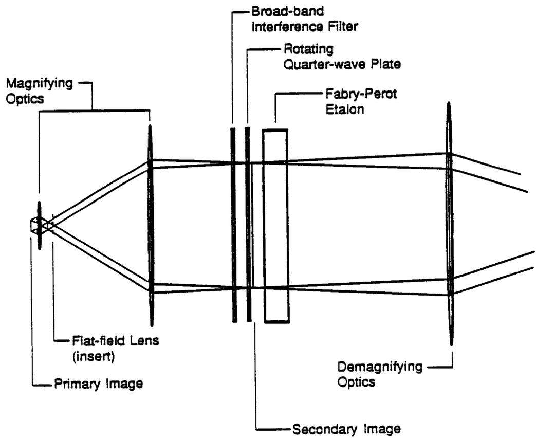
Figure 1. The modulator section of the Imaging Vector Magnetograph. Vertical exaggeration is 5:1.
