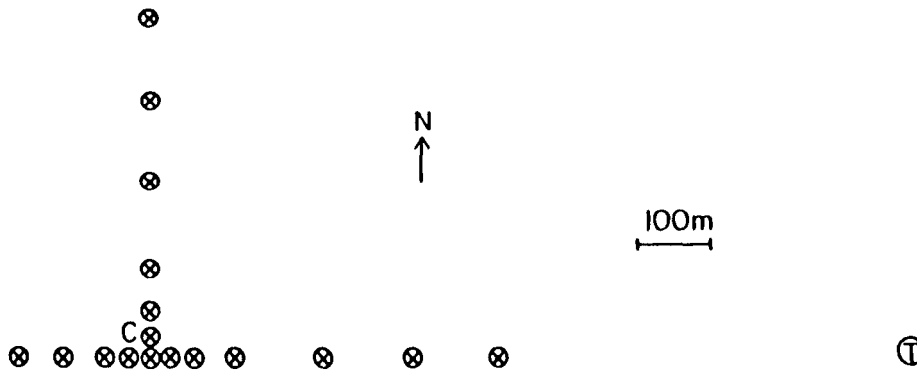
Interferometer configuration, showing the possible locations of the 27 m antennas (x) relative to the 40 m telescope (T) and the control room (C).
