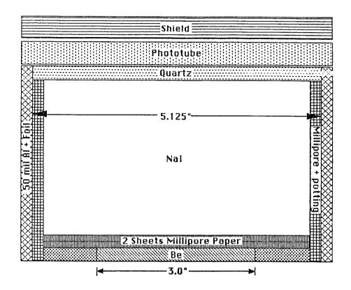
Figure 1. Model for Monte Carlo simulation of the BATSE spectroscopy detector, showing some of the materials and geometry. Flux may be incident from any direction, since the BATSE experiment contains eight of these modules oriented in the directions normal to the faces of a regular octahedron. The nominal view direction is downwards on this sketch.
