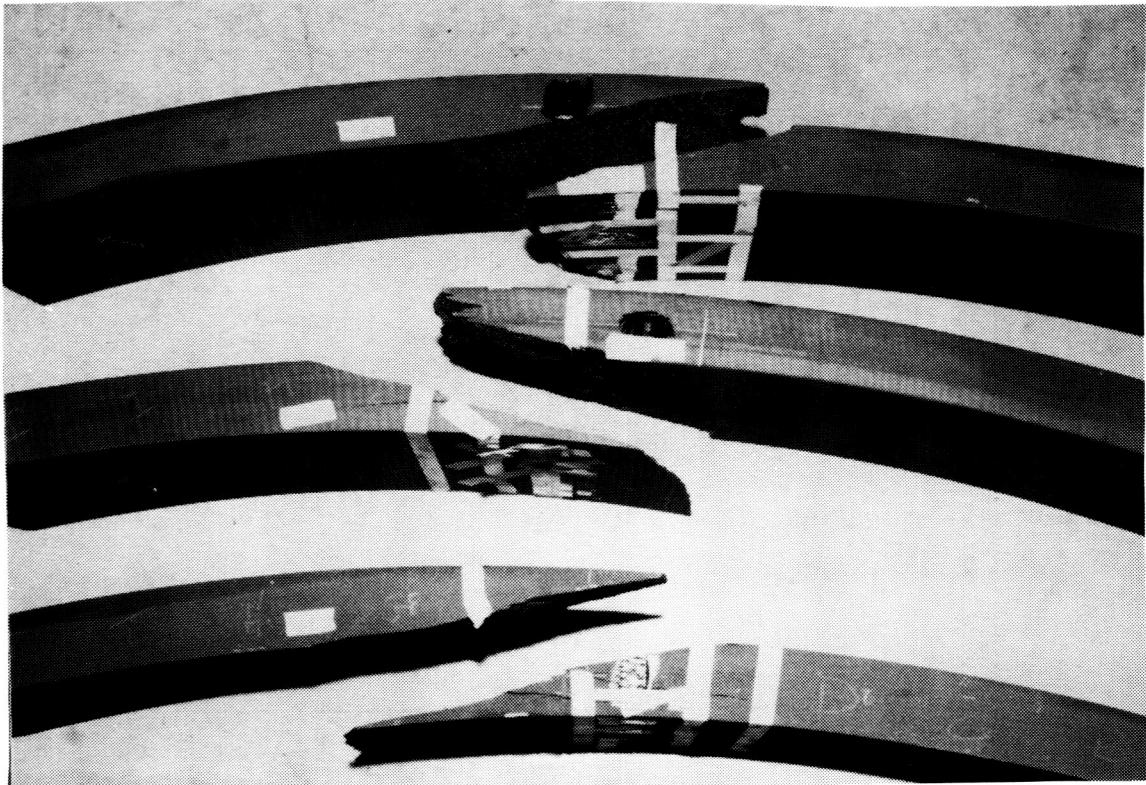
Figure 22. SRB 30-in. segment cyclic load test, uncycled specimens.
