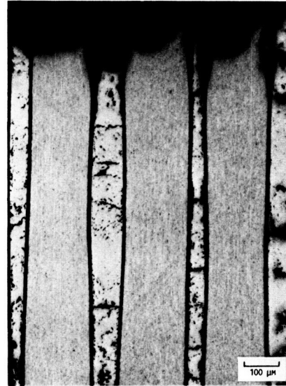
FIGURE 22. - FRACTURE SECTION OF ST300/Nb + 1Zr CREEP RUPTURE SPECIMEN.
