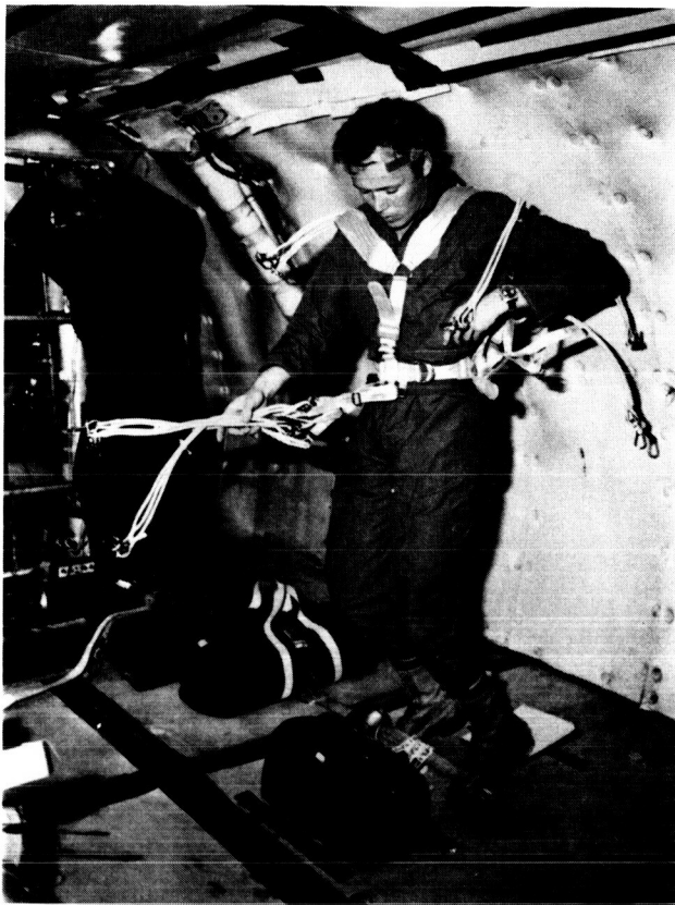
Figure 1. Handling test of torso harness and bungee cords used on Spacelab missions SL-1 and D-1.
