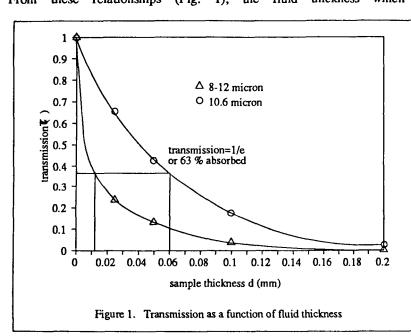
incoming radiation is found to be 0.200 mm and 0.256 mm for the 8-12µ region and 10.6 wavelength respecively. Therefore, it is concluded that the "surface" the imager "sees" is 0.200 mm thick. The fact that the CO<sub>2</sub> laser radiation penetrates deeper than this is advantageous. If the situation were reversed, the temperature indicated by the imager would be an average over a region where a much larger temp-
