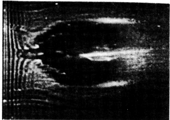
Figure 15. Generation of an Artificial Event in a Laminar Boundary Layer Using Two Suction Holes. Top View is Visualized Using Hydrogen Bubbles and a Horizontal Sheet of Laser Light.
