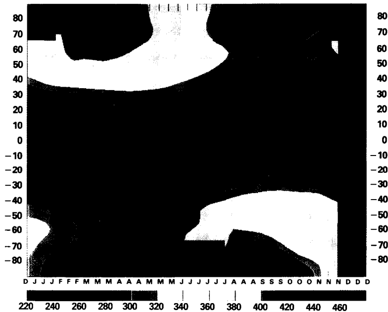
Figure 6 (a) Zonal mean values of total O_3 (Dobson units) retrieved from TIROS-N HIRS2/MSU soundings for each 1/3 of a month for the period Dec. 21-31, 1978 to November 1-10, 1979. (b) As in (a) but for O_3 derived from TOMS soundings.
