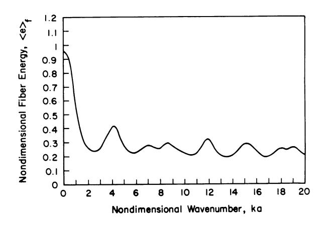
Fig. 3 Nondimensional fiber energy,  $\langle e \rangle_f$  as a function of nondimensional wavenumber ka for  $r_p = 1.5$ , and  $r_{\mu} = 7.5$ .
