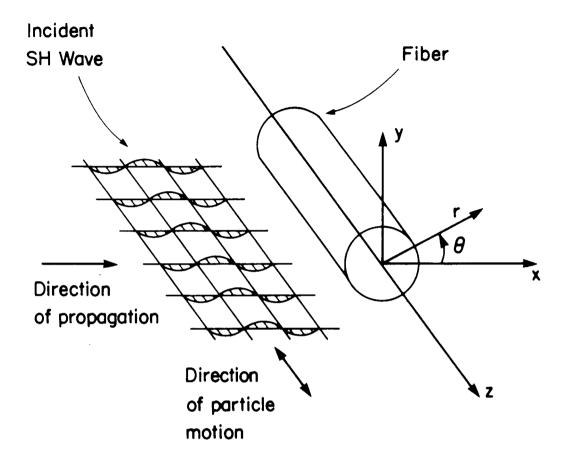
Fig. 1 Elastic fiber embedded in infinite elastic matrix containing incident SH wave.
