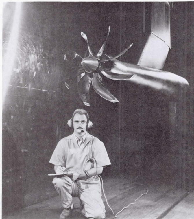
Figure 4. - SR-3 propeller model with 45^{\circ} - swept blades installed in NASA Lewis 10 - by 10 - Foot Supersonic Wind Tunnel.
