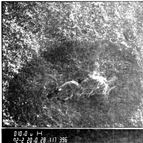
Figure 10.--EDX and SEM Photos of Fractured Bar 4079 Showing Dark Inclusion and Surrounding Patch.
