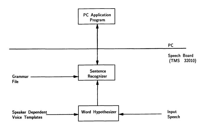
Figure 2 - LR 2000 Block Diagram
