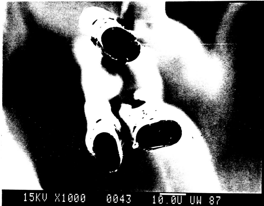
Figure 12. Scanning Electron Microscope Photograph of a Group of Nextel 312 Fibers.
