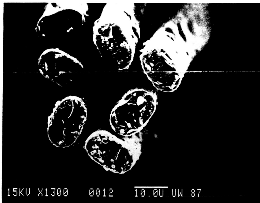
Figure 13. Scanning Electron Microscope Photograph of a Group of Nextel 380 Fibers.
