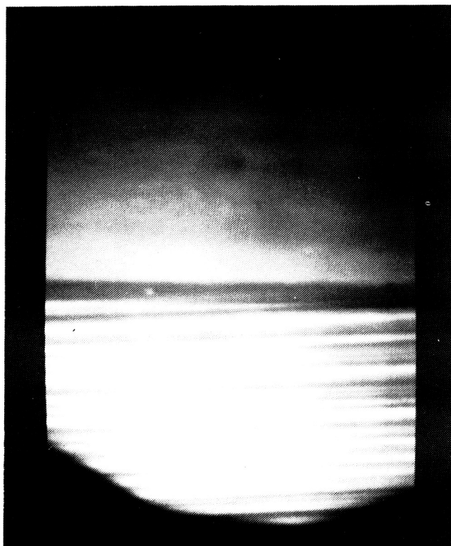
Figure 7. IR micrograph showing growth striations below the regrowth boundary and evidence of uniform growth above the boundary.
