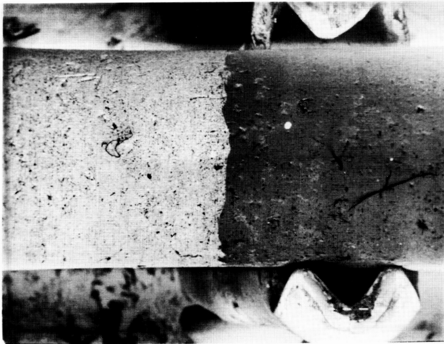
Figure 3-A Pb-Zn Interface Flight Specimen No. 10 15X
